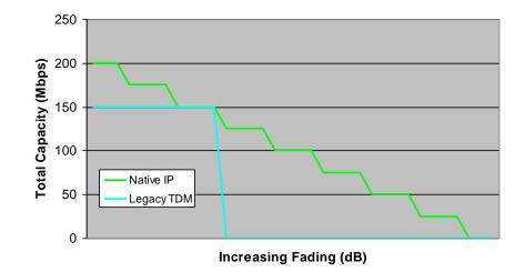
In other words, the native IP enables granularity in the traffic, so that transmission is not just ON/OFF depending on fading (as it happens in TDM systems), but continuously liaising across the multiple classes of priority pertaining to the several modulation formats, and gradually reducing the capacity accordingly as soon as the fading increases.
