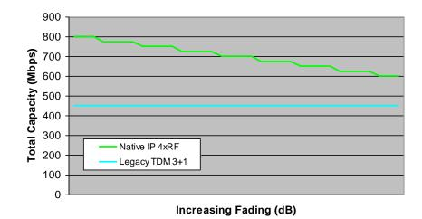
Even if we consider that the TDM system may use some Occasional TDM traffic function (meaning transmitting some low priority TDM traffic on the protection channel), the situation does not improve much, as shown in the following figure.
