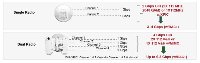
Figure 1: Single vs. Dual Carrier Configuration
