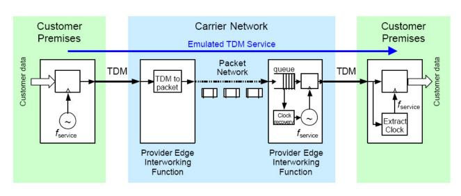
The TDM service frequency *fservice* at the customer premises must be exactly reproduced at the egress of the packet network. The consequence of a long-term mismatch in frequency is that the queue at the egress of the packet network will either fill up or empty, depending on whether the regenerated clock is slower or faster than the original. This will cause loss of data and interruption of the service.
