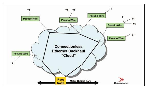
An Ethernet networking benefit for TDM transport is that virtual 1:3 cross-connecting can be realized in the aggregation of T1 tail circuits without additional equipment. Additionally, the connectionless nature of Ethernet allows highly flexible deployment of T1 circuits anywhere in the network, since Ethernet allows the re-targeting and re-configuration of available network capacity with great ease.
