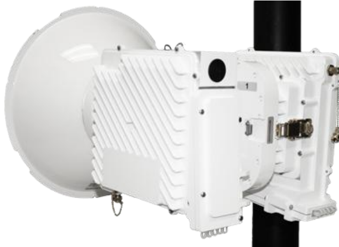
Figure 1: One end of a typical 2+0 XPIC point-to-point microwave radio link with traditional single-carrier transceivers that provides 1 Gbps data rates.
